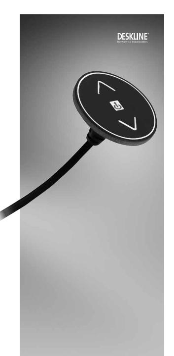
The DPH Desk Panel is a small, compact and userfriendly panel, which can be used for all kinds of height adjustable desks from heavy-duty workstations to standard office desks. The desk panel is made of foil and has the basic up and down function for adjusting a desk. Because of a small size the DPH is very easy to integrate in the design of the tabletop of a desk, kitchen table or similar. Besides availability in either black or white, the DPH can be customised.
